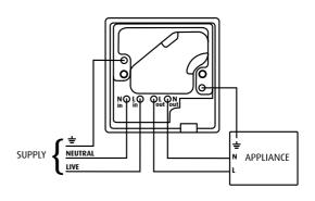
Remove cut-outs before fixing the box. Where appropriate drill the box to provide close fitting entry for cables and heat-resistant flexible cords. Take care to remove sharp edges.
