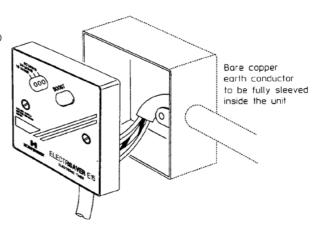
THE ELECTRISAVER SHOULD BE KEPT IN ITS SEALED PACK UNTIL ALL DUST AND DEBRIS HAVE
